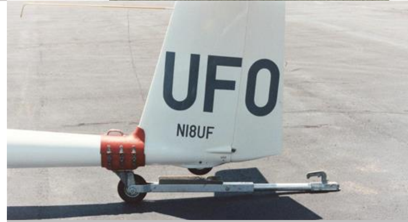
Tow bar and wing wheel allow you to grid yourself. Using just a rope requires 2+ people.
